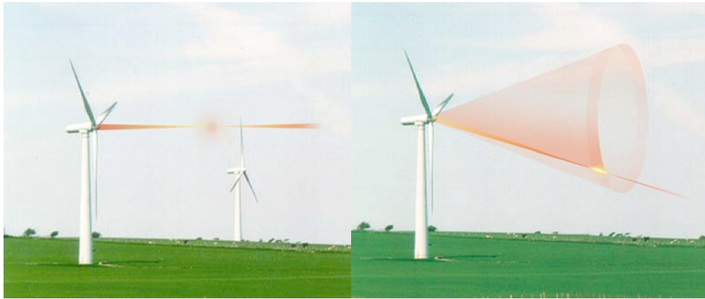
Figure 7: Wind turbine inflow measurements using hub-mounted LIDAR .
