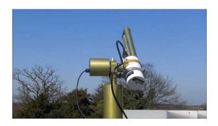
Net Radiometer: measures the difference between incoming and outgoing radiation.
