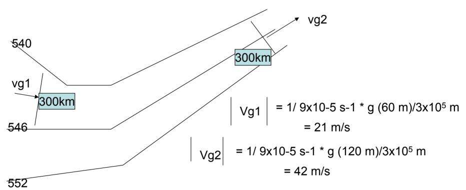
Direction is parallel to height lines or from 300° for Vg1 and 250° for Vg2
