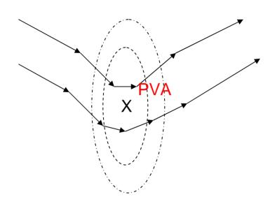
Air travels through the pattern (moves faster than the trofs/ridges) and must slow down its spin (vorticity) as it exits the wiggle/trof. To do this, it must diverge like an ice skater spreads out their hands to slow down their spin.
