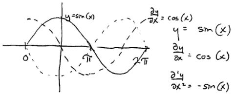
We see that the local maximum of y = sm(x)13 indeed located where  $\frac{\partial y}{\partial x} = cos(x) = 0$ , i.e. at  $x = \frac{\pi}{2}$ , and that  $\frac{\partial^2 y}{\partial x^2} = -sm(x) = 1$  at  $x = \frac{\pi}{2}$ . Then if a jet streak is a local maximum of the wind speed, we expect that the jet streak is where
